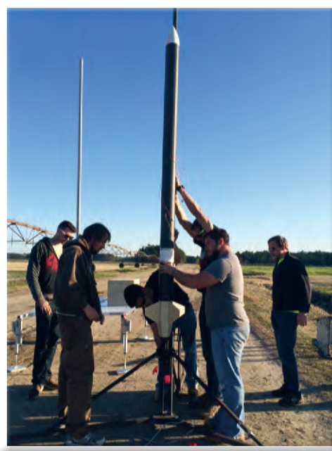
The team is preparing the on-board altimeters to record flight apogee and data.
